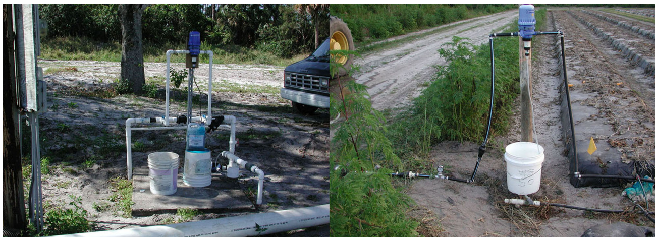
Figure 1. Example of injection loops using a Dosatron (left) or a Mazzei injector (right).
