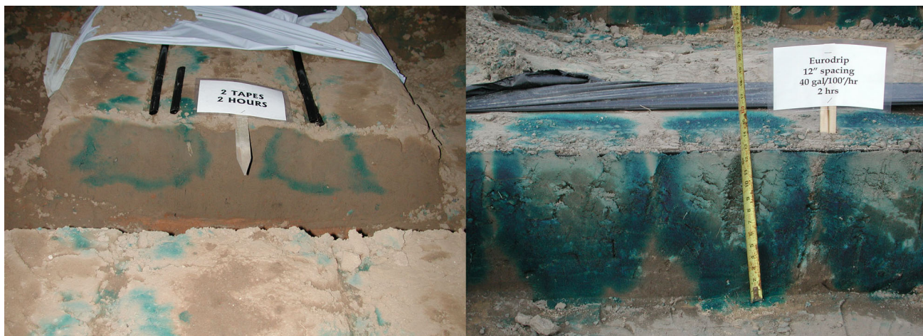
Figure 3. Sample dye pattern on transverse (left) and longitudinal (right) sections.
