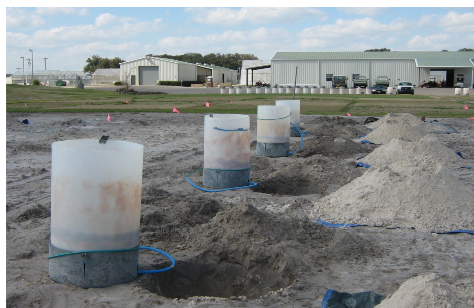
Fig. 1. Lysimeters along with excavated pits
